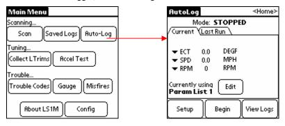
This is the main Auto-Log screen. Here, you can specify three parameters to "keep an eye on" while you're waiting for the logging to start. Click on one of the parameters on the left (ECT, MPH or RPM in this picture) and a window pops up with a list of all the parameters that are available.
